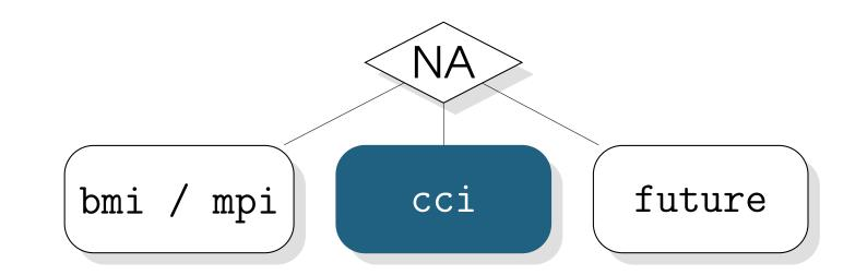
bmi / mpi: TCP/IP, IB cci: TCP/IP, IB, Cray GNI, shared memory
